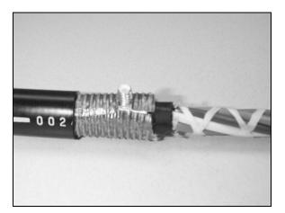
Figure 10 - Install bottom half of bond clamp.
