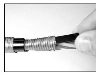
Figure 19 – Insert the plastic guard.
