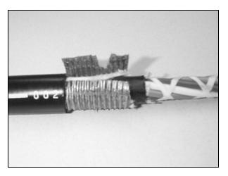
Figure 14 – Cut a slot in armor.
