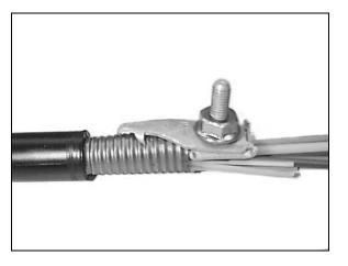
Figure 5 - Install the top half of the bond clamp.
